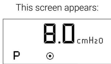
**Pressure** set by the physician (corresponding to the pressure prescribed when the device is operating).
