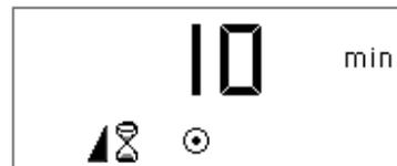
**Ramp time** set by the physician (time the device takes to reach the prescribed pressure when starting from the comfort pressure).
