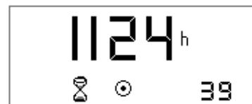
Value of the **hour counter** (device operating time). The value displayed on the right below represents the minutes.
