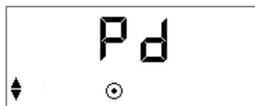
Selection of the pressure displayed: **prescribed pressure Pd** or **actual pressure Pr** (estimated at the mask). The selection is done by pressing the button
